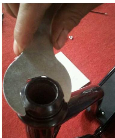
To fix locknut with the help of the wrench and ensure that it is tightly fixation.
