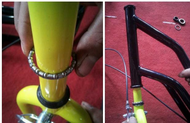
Please pay attention to the direction of thread bearing shows by the photograph then to return the fork by taking care well that bearing ball is in housing envisaged has its effect.
