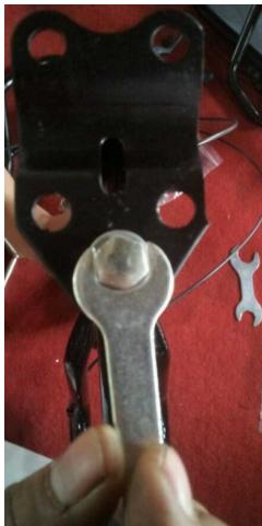
Place the bracket in the column steering, using the wrench to tighten the long screw.
